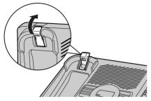
2 Press the tabs in the direction of the arrows (①), then remove the wall mounting adaptor (②).
